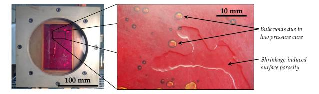
Figure 1: Lab-scale RTM with neat resin sample cured at low pressure, containing both types of voids.
